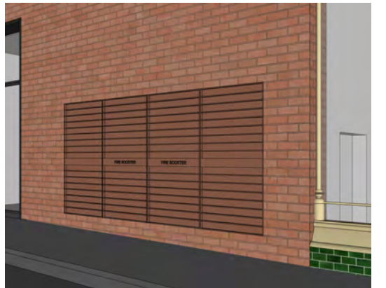
07 - FIRE BOOSTER, VALENTINE ST VIEW
